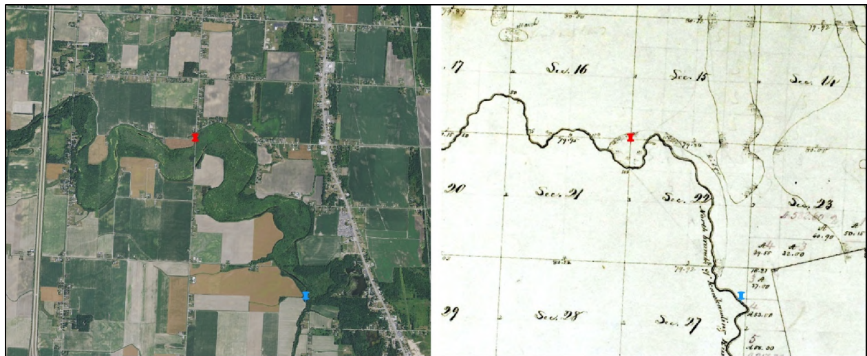
Figure 3: Comparison of 2012 aerial photograph with the 1843 plat map. The red pushpin indicates the point described by the surveyors as swampy and marked as such on the 1843 map.
